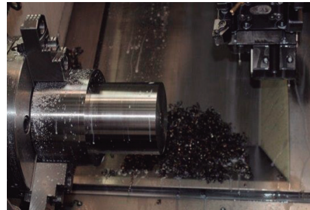
Workpiece material: Low-alloy steel, Ck45 (200 HB)
